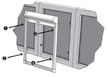
Firmly press the frame down onto each bracket. Fit one side at a time for an easier installation, 1, 2, 3, 4.
