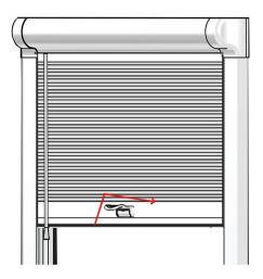
To release the blind, tilt the handle forwards. The blind is then free to be raised and lowered.
