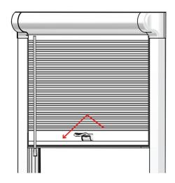
To lock the blind into position, tilt the handle backwards.
