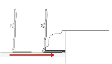
Push the bracket firmly into place between the glass and the rubber seal.
